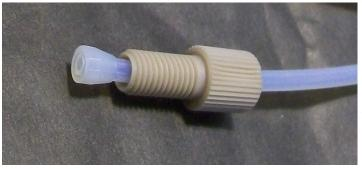
Unlike many compression fittings for metal tubes (such as Swagelok), the ferrule must be installed "backwards". Before assembling the fitting, make sure that the tubing end is squarely cut by a new razor blade and is flush with the broader ferrule end.
